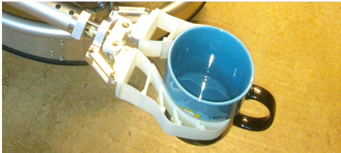
Fig. 5. Fin Ray Effect: gripper automatically wraps around object without additional actuation
