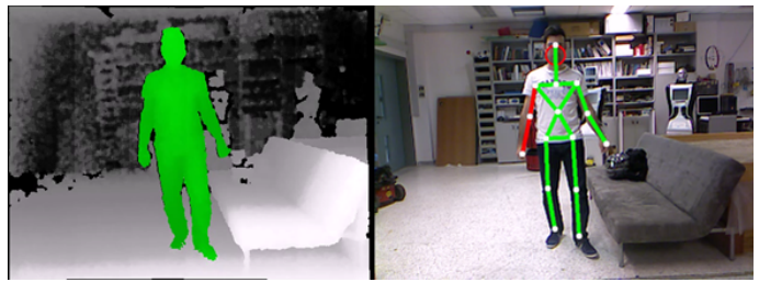
Fig. 13. Vision-based 3D human observation. 3D human body detection is performed identifying a human body (green color-left depth image) and segmenting it from the background in the observed depth scene. Subsequently, 3D pose estimation is applied on the segmented body data to fit a 3D skeletal model of the human body (right color image) and estimate the 3D position and orientation of 15 body joints (white dots) and infer the body limbs (red/green lines).
