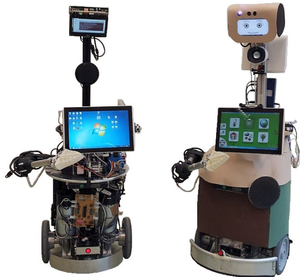
Fig. 1. The “naked” Hobbit robot (left) and the Hobbit robot (prototype 1) used for the first round of user trials (right) in Austria, Greece, and Sweden.
