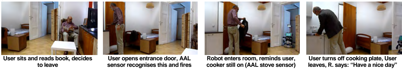
Figure 3: Still pictures from video demonstration of the safety / stove reminder scenario in AAL laboratory
