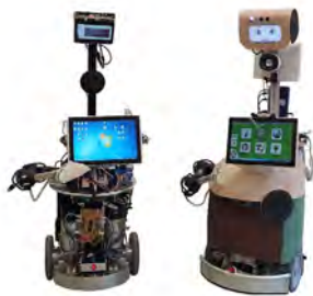
Figure 1: The HOBBIT robot without (left) and with cover as used during the first user trials (right) [3]
