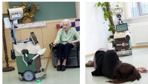
Fig. 4: Three of the six robot tasks: bring an object, pick-up an object from the floor, and detect an emergency situations (here acted out by a young colleague in the user trials).
