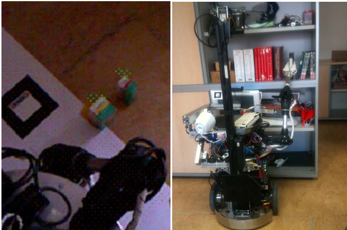
Figure 6: View from camera in robot head and PT1 robot arm taking on object.
