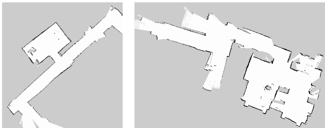
Figure 1: New maps built with the two Hobbit prototypes PT1 at TUW, including long corridors.
