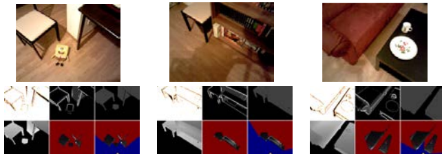
Fig. 2. Top: RGB scenes. Bottom: preprocessing for obstacle avoidance. For each scene, from left to right and top to bottom: confidence map, relative gradient values of the lower resolution disparity image with respect to the vertical gradient of the line corresponding to the floor, points outside a disparity value band around the floor disparity are labeled as obstacle points, projection onto the floor plane, projection labeled, virtual 2D laser scan obtained by raytracing the labeled grid.
