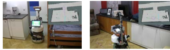
Fig. 7. A previous prototype of the Hobbit robot (with the same sensor configuration as described here) navigating between predefined places.
